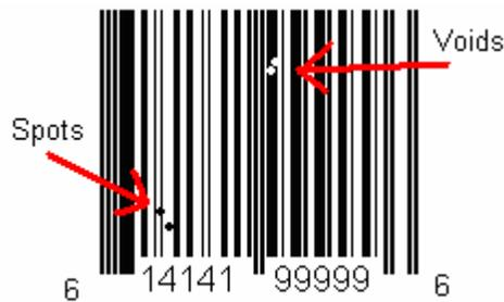
Figure 6.22 – Symbol with defect failure from spots and voids
