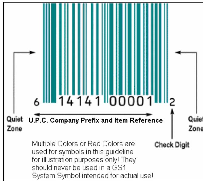
Figure 5.1 – The GTIN-12 ID number and the UPC-A symbol
