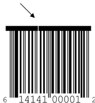
Figure 6.4 – Line detecting print head element burnout
