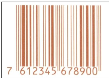
Figure 7.2 – Symbol with a failing minimum reflectance
