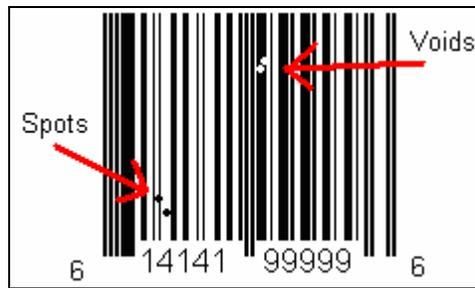
Figure 7.4 – Symbol with defect failure from spots and voids
