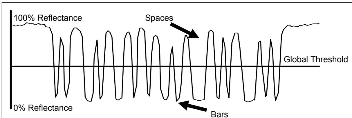
Figure 7.1 – Bar code represented in a Scan Reflectance Profile
