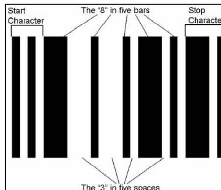
Figure 5.9 – ITF-14 encoding of a two-digit pair
